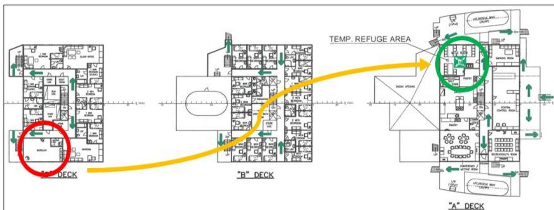
**Figure 1.** Layout of escape route from Musolla to the muster area.
