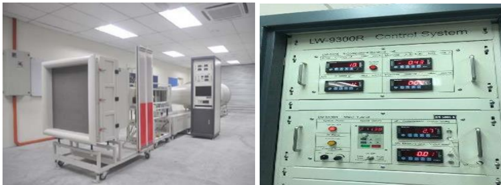
Figure 4 Overview of LW-9300R Wind Tunnel (left) [19] and monitoring display (right).
