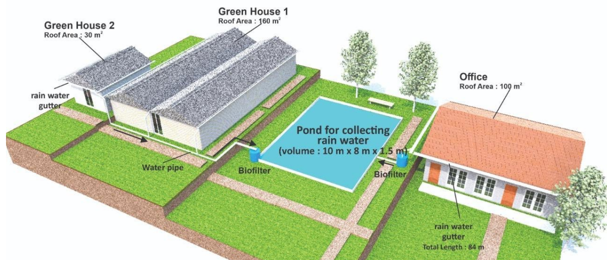
Figure 3: Technical design for rain water collecting system
