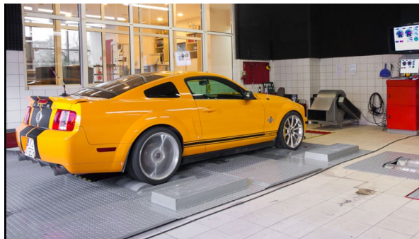
Figure 23: Experiment using chassis dynamometer conducted in laboratory
