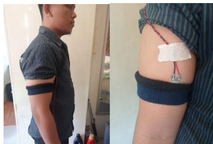
Figure 3: Placement of sensor attached using double-sided tape and armband
