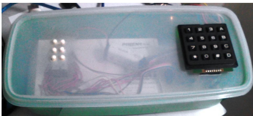
Figure 8: All Braille pins rise up after the voltage is supplied
