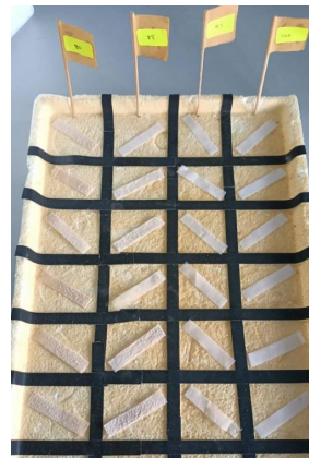
Figure 2: Samples arrangement for UV Degradation Test
