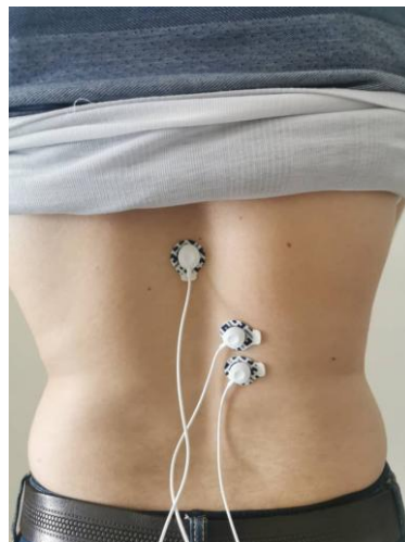
Figure 2: Electrode placement (as per SENIAM recommendation)
