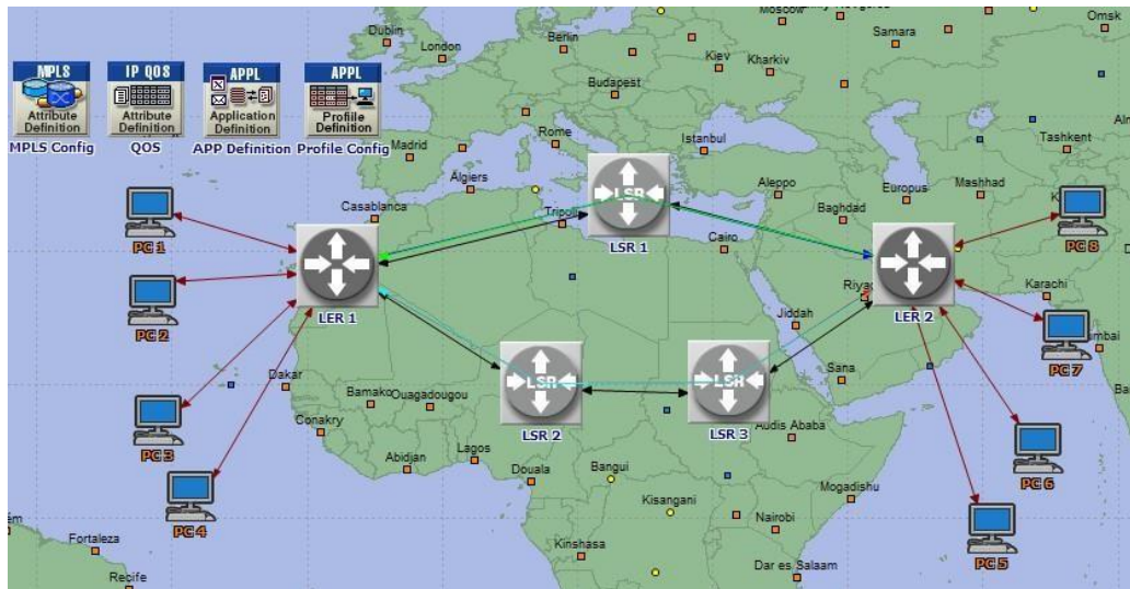
Figure 1: Network Design with MPLS and MPLS-DiffServ
