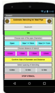
Figure 4: Graphical User Interface (GUI) for Automatic Stencil for Steel Pipe in Android OS.
