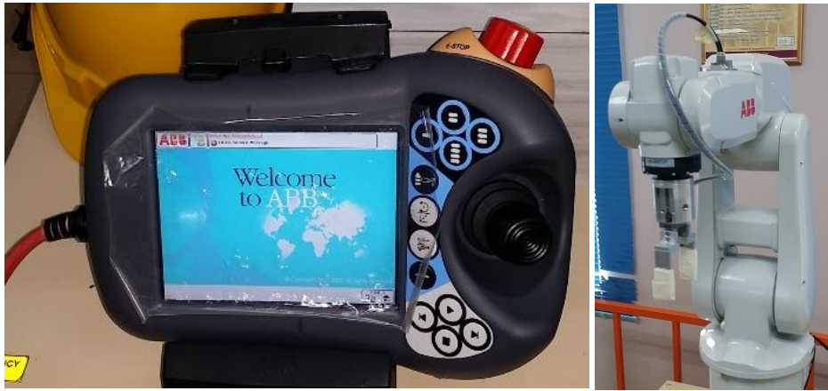
Figure 6: ABB Robot's controller (left) and ABB Robot main body (right)
