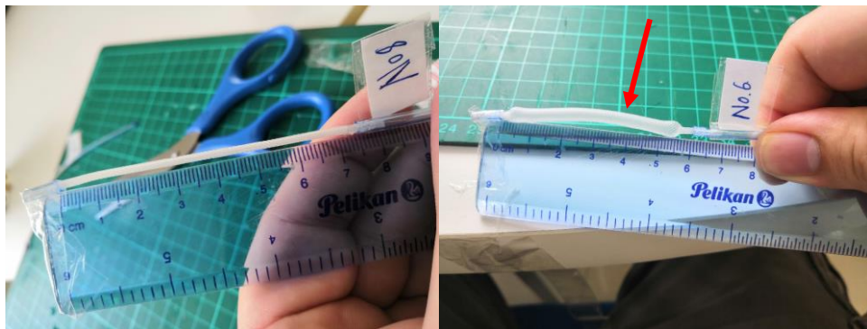
Figure 6 Thin McKibben Length Contraction Testing and Measurement Setup
