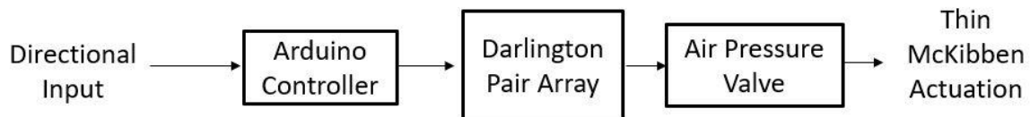
Figure 4 Open Loop Block Diagram of the Robotic Eye Control System
